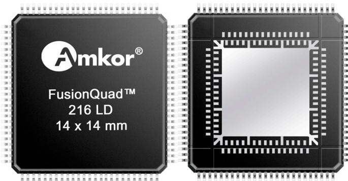
FusionQuad™ offers a unique blend of excellent electrical and thermal performance in a miniaturized cost-effective leadframe plastic package. The unique footprint of FusionQuad™ allows for the use of low cost printed circuit boards in the end application due to the space available for coarse routing vias between the bottom lands and the outer peripheral leads.
