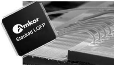
Die stacking technologies have been demonstrated up to 24 high stacks, however, most stack ups greater than 9 devices high use a combination of die and package stacking technologies to address complex test, yield and logistic limitations.
