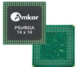
Amkor is now entering the second generation for PoP applications where new memory architectures required in mobile multimedia applications, demand higher density stacked interfaces in combination with PoP mounted area and height reductions. The current PSvFBGA and PSfcCSP structures limit the ability of the memory interface to scale in density and pitch, thus a new bottom PoP structure was needed.
