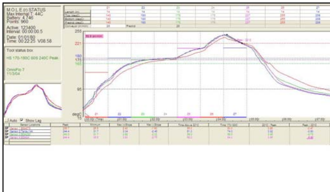
Figure 6. Soak profile for SAC305 alloy. Soak time is 60 seconds at 175 C. Peak temperature is 235-240 C.
