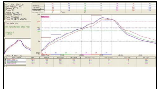
Figure 4. Ramp profile for SAC305 alloy. Ramp rate is 1.2 C/sec. Peak temperature is 230-240 C.
