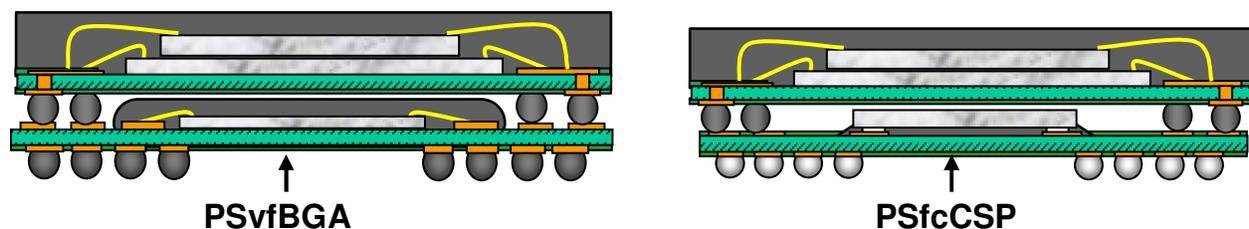
**Figure 1:** 1<sup>st</sup> generation of PoP stacks. PSvfBGA with center gate mold and PSfcCSP with exposed flip chip die.
