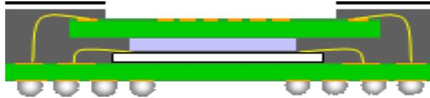
**Figure 3:** Dual laminate sandwich PoP structure.
