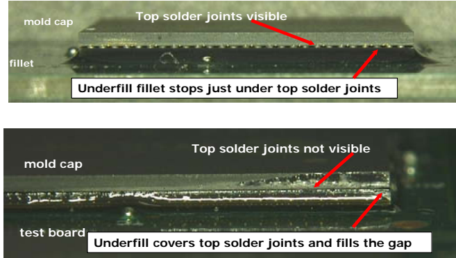
Figure 14: Cross sections of underfill coverage.
