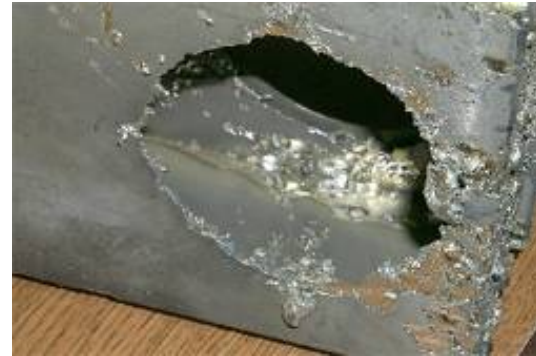
Figure 2. Stainless steel flow duct corroded by tin-rich solder alloy. Stainless steel will degrade after 6 – 12 months exposure to lead-free solder.
